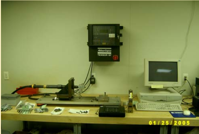
An RS Technologies manufactured Torque Tension testing station to ensure compliance to specific lubricity requirements
